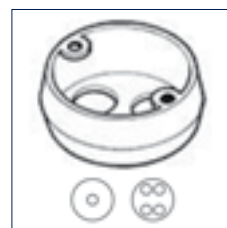
ATBLI142 Medium Steel 1 Hole or 4 Knockouts 29mm Deep x 63.5 mm Internal Diameter
